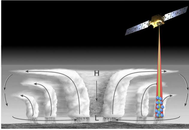
**Figure 4.** Artistic representation of the concept of laser-induced condensation for tropical cyclone control (not to scale). The red and green laser beams represent the femtosecond pump beam and nanosecond probe beam, respectively.
